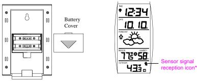
\* When the signal is successfully received by the Weather Station, the icon will be switched on. (If not successful, the icon will not be shown in LCD) So the user can easily see whether the last reception was successful (icon on) or not (icon off). On the other hand, the short blinking of the icon shows that a reception is being done now.
